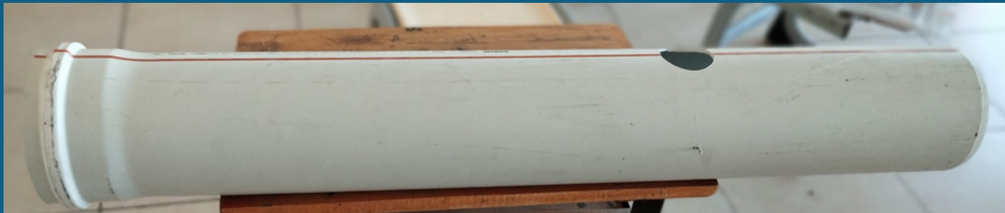
PVC pipe for telescope tube
